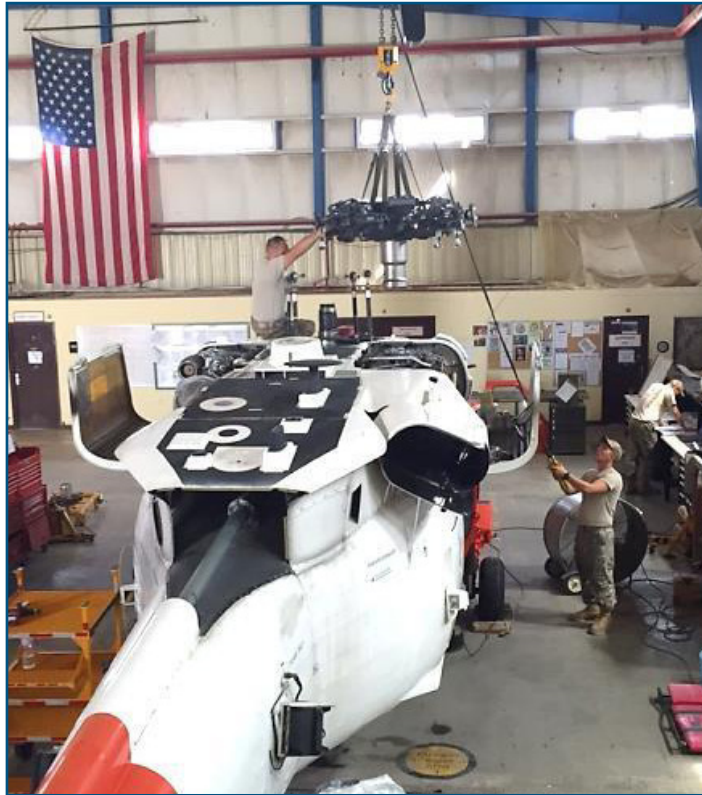
First Sgt. Douglas Krol (left), 1108th AG, and Spc. Daniel Burke (right), Aviation Company, Task Force Sinai, re-install the main rotor head on a UH-60 Black Hawk July 27 at North Camp, Sinai, Egypt, during a preventative maintenance inspection cycle.
