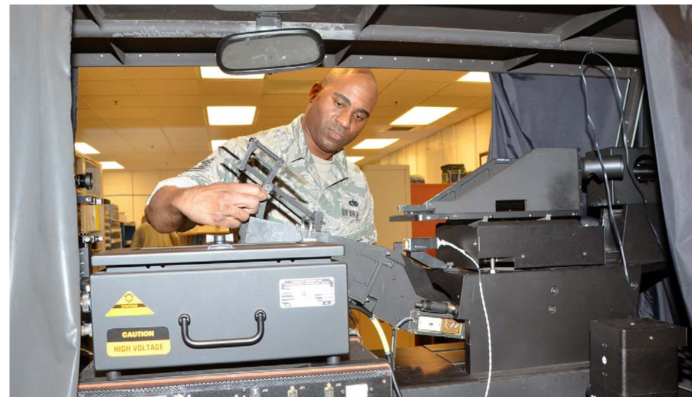
Bottom: Tech. Sgt. Sadiki A. Givens places the Heads-Up display into the Display Unit Test Set Nov. 6. The sight lines of the display must be calibrated to the center of the screen. (U.S. Air National Guard photo by Master Sgt. Betsy J. Winstead)
