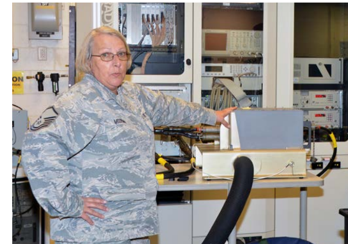
Top: Master Sgt. Alice M. Moorman points out the Central Interface Processor of the C-17 Automated Test Equipment system Nov. 6. This is in preparation for final testing of the repaired unit. (U.S. Air National Guard photo by Master Sgt. Betsy J. Winstead)
