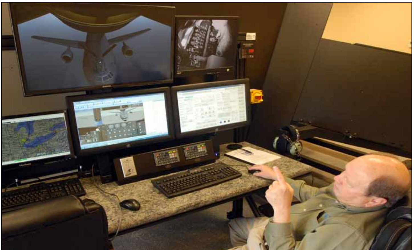
William Eger, an equipment specialist for simulator certification, changes the mission environment in the Boom Operator Simulator System to present the trainee with an obstacle to overcome during a demonstration April 16 at Key Field. The BOSS at Meridian is the first of 17 to be delivered to the National Guard.
