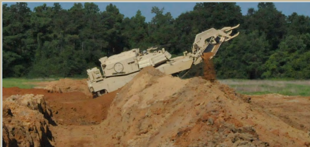
An Armored Breaching Vehicle mine plow from Charlie Company, 155th Brigade Support Battalion clears a tank ditch for other vehicles to pass through on July 25 at the Camp Shelby Joint Forces Training Center. The "ABV" has a plow that clears a path through a minefield enabling other vehicles to safely pass through. (Army National Guard photo by Staff Sgt. William Hill, 155th ABCT) Inset, An AH-64 Apache of the 149th Aviation Battalion, based in Tupelo, makes a low pass over an M1A2 SEP v2 from the 155th ABCT during a Combined Arms Live-Fire Exercise on July 23. (Army National Guard photos by Staff Sgt. William Hill, 155th ABCT Public Affairs)
