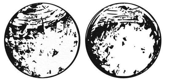
Figure D-4. Fatigue failure, no stress, and high stress concentration
